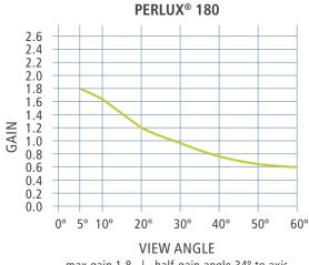
max gain 1.8 | half-gain angle 34° to axis
