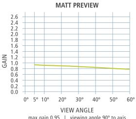
max gain 0.95 | viewing angle 90° to axis
