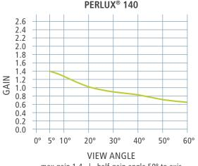
max gain 1.4 | half-gain angle 50° to axis
