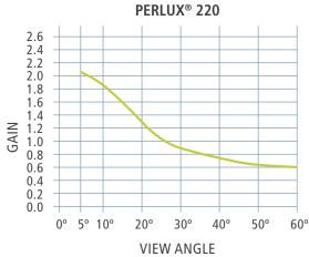
max gain 2.2 | viewing angle 25° to axis
